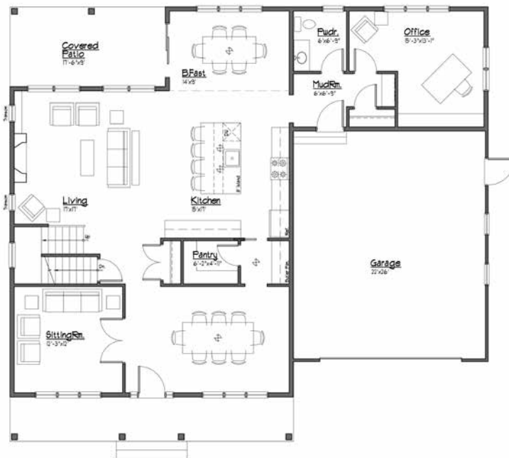
FIRST FLOOR PLAN SCALE: 1/4"=1'-0" 1558 Sqft. - First Fl. 1679 Sqft. - 2nd Fl. 3171 - TOTAL
